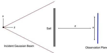
Fig. 5: Defining the observation plane with respect to the lightsail
