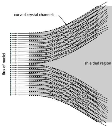
Fig. 6: Deflection of high energy ion using a series of bent silicon crystals
