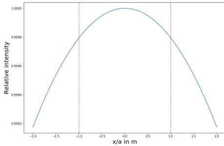
Fig. 4: Diffraction profile of a circular stop for incident Gaussian beam:  $\lambda = 10^{-6}$ ,  $\omega_f = 0.5$  m, aperture  $a = 0.5$  m, distance  $z = 10^8$  m
