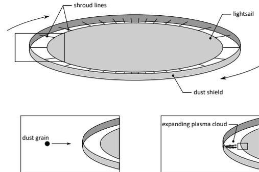
Fig. 7: Edge-on sail orientation with dust shield
